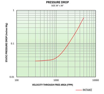
Tested per AMCA Standard 500-D using test set-up.
